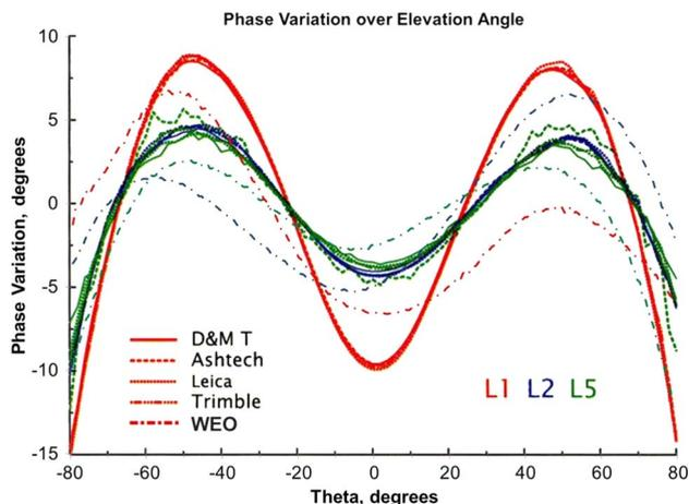
Fig. 2. Comparison of measured phase variation of five high-performance GNSS antennas.
