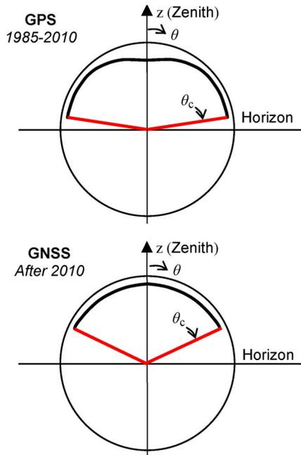
**Fig. 1. Ideal antenna gain patterns for GPS antennas (1985–2010) and GNSS antennas (after 2010).**
