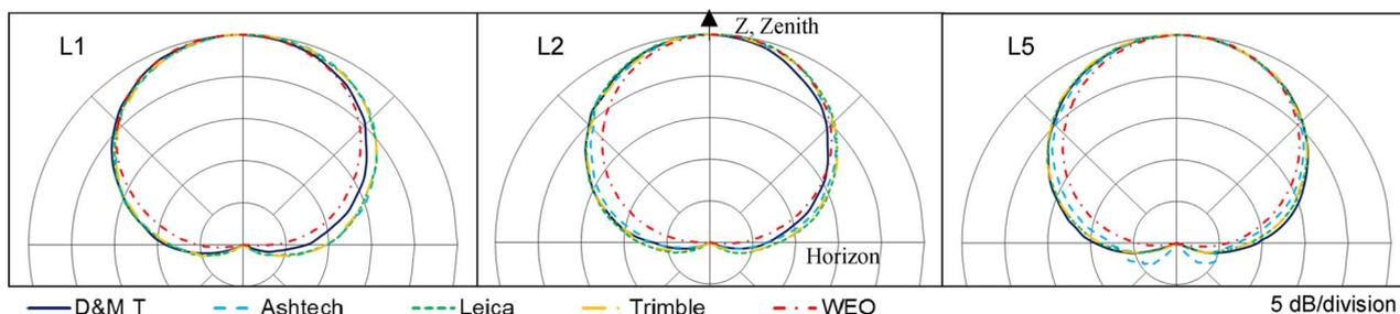
Fig. 3. Relative gain pattern for five high-performance GNSS antennas showing different amenability to higher cutoff angle  $\theta_c$ .
